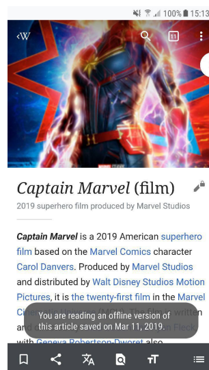
Figure 5.9: Although the device is actually connected to the internet, not granting permission ACCESS_FINE_LOCATION prevents the app from accessing the network. The app continues working with cached data only.
