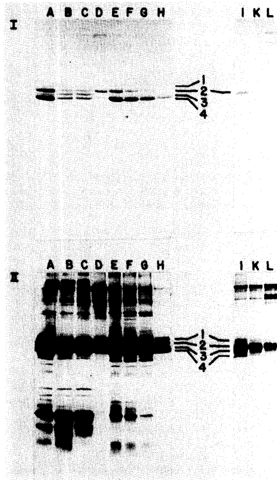
Fig.2. SDS gel electrophoresis of fractions obtained from the affinity column of fig.1: (A) hydroxylapatite eluate; (B) fractions 7-8; (C) fractions 9-12; (D) fractions 35-40; (E) fractions 41-42; (F) fractions 43-44; (G) fractions 45-46; (H) fractions 47-48. (I,K,L) Taken from a separate gel: (I) fractions 39-40; (K) fractions 37-38; (L) fractions 35-36. I, Coomassie blue stain; II, silver stain, performed after Coomassie blue staining.
