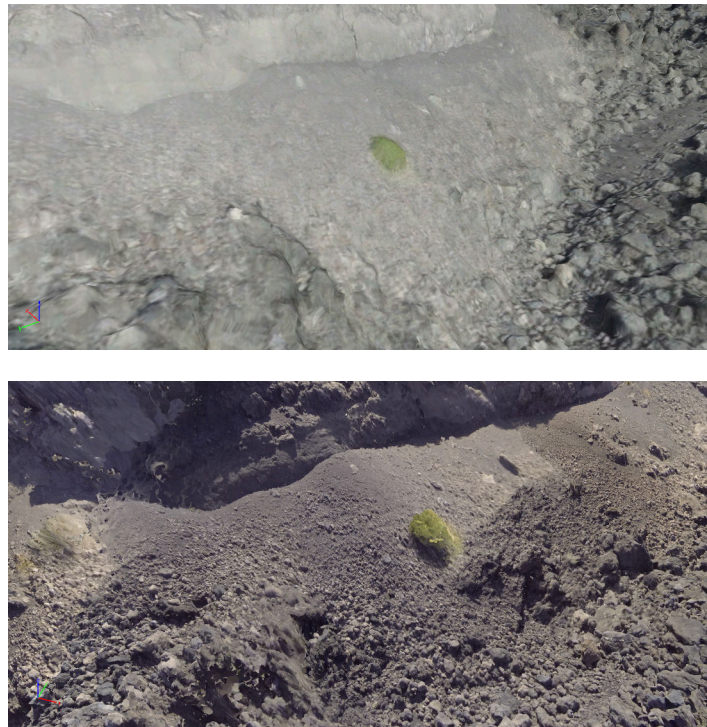
Figure 31. On-field test: a comparison of the 3D meshes of the lava flow reconstructed by Pix4D mapper. The image on the top shows the results obtained by using the images acquired during the first flight, at high altitude (20 m). The image at the bottom shows the same area reconstructed by using the images acquired during the flight at low altitude (5 m).
