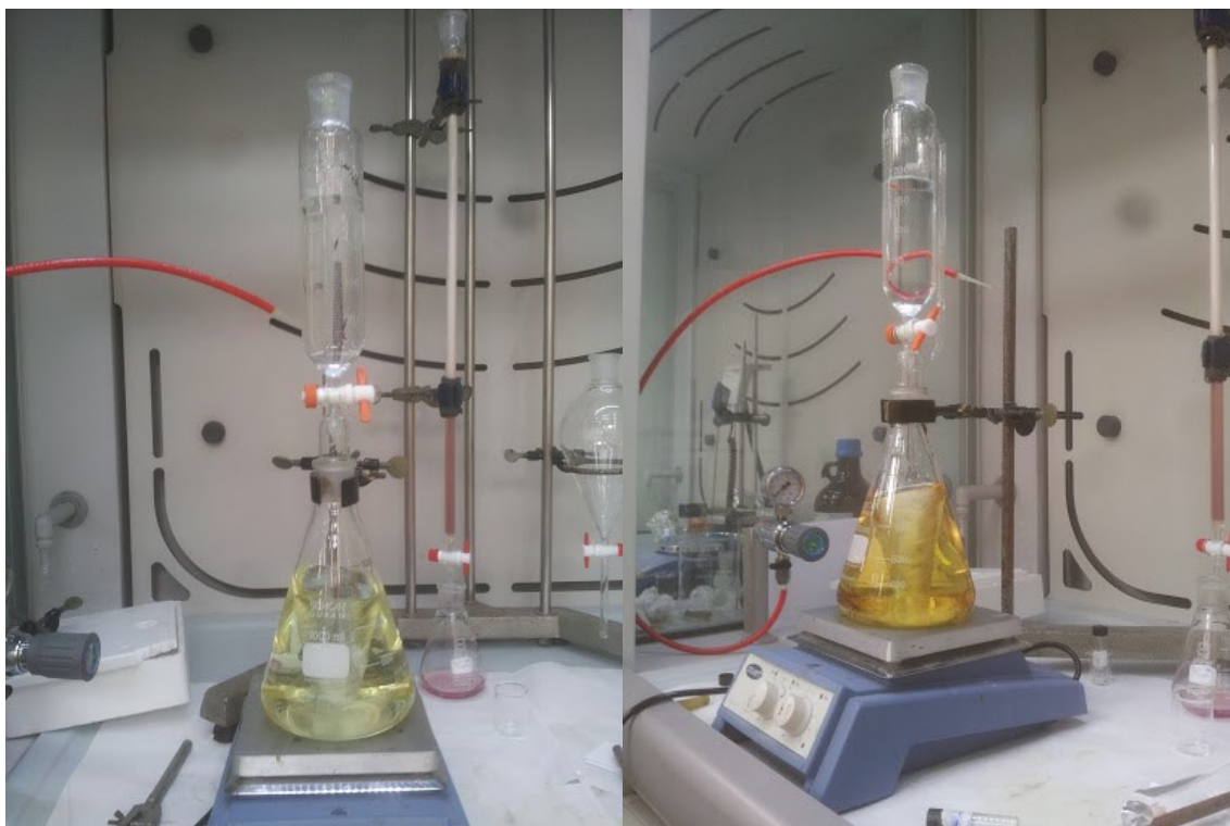
Figure 3.3.3: Synthesis of silver nanoparticles (AgNPs). In the photo you notice the progress of the reaction: the photo on the left was taken about 2-3 minutes after of reaction, the photo on the right about 10 minutes after the reaction.
