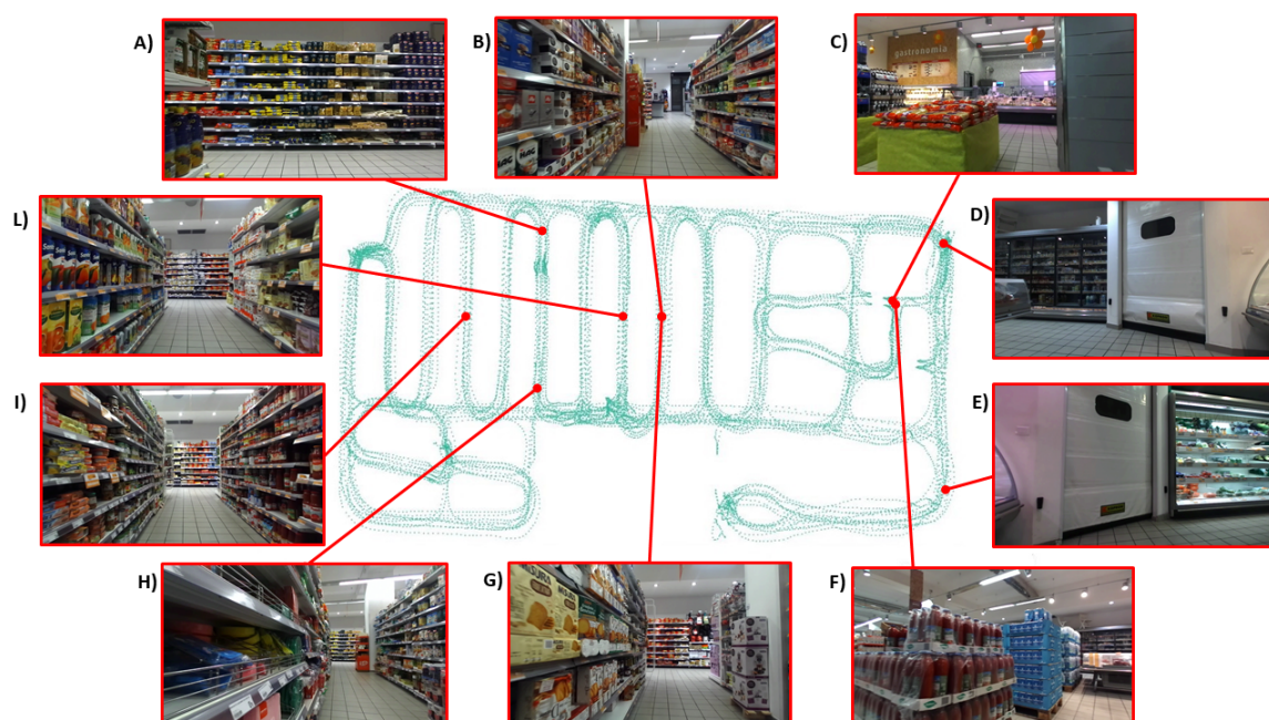
Figure 4.3: Confounding couples of frames for pose regression task: A) and H) images that frame the same shelf at different scale, B) and G) frames in the same corridor with opposite direction, C) and F) frames with same position but different orientation, D) and E) images, with different positions, frame similar structure, L) and I) images of two different corridors with high visual similarity
