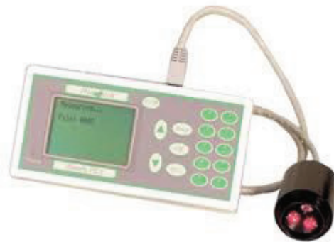
Figure 5 – The continuous excitation chlorophyll fluorimeter used to determine the chlorophyll fluorescence on the Miscanthus leaves during the heat stress experiment.
