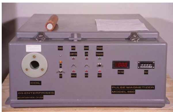
Figure 33. The 2G pulse magnetizer, the field can reach up to 2.7 T
