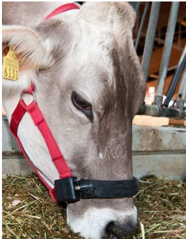
Figure 3. RumiWatch noseband sensor.
