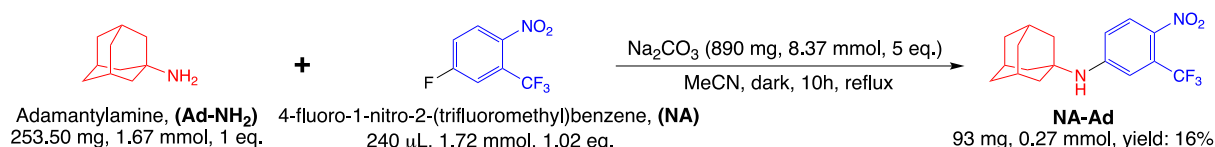
Figure 86: Synthesis of nitroaniline-adamantane (NA-Ad) from adamantylamine (Ad-NH 2 ) and a nitroaniline (NA) derivative.
