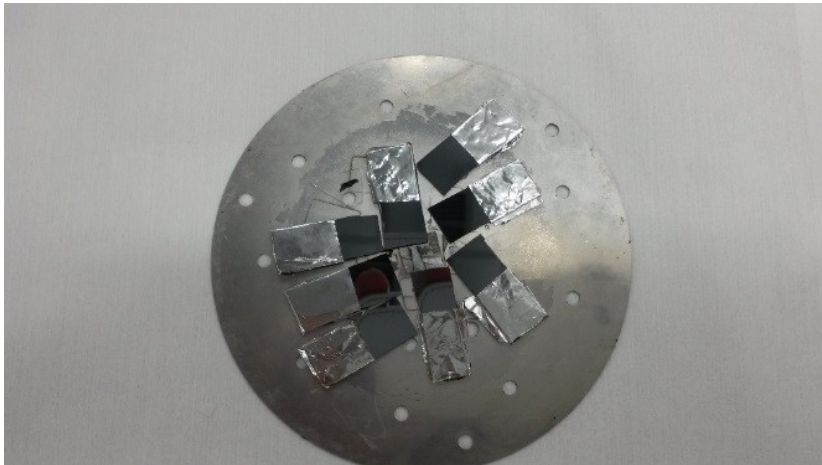
Figure 2.2.4 Picture of eight Si (100) n + doped electrodes mounted on the rotation stage. The portion of the electrode masked by an aluminum foil was not metalized.
