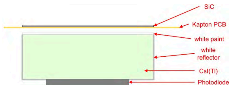
Figure 10. Scheme of the elementary telescope cell of the NUMEN Particle Identification Detector.
