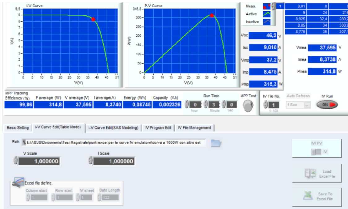
Figure 27. PV modules model validation, first session: emulation of a PV module through the DC power supply software
