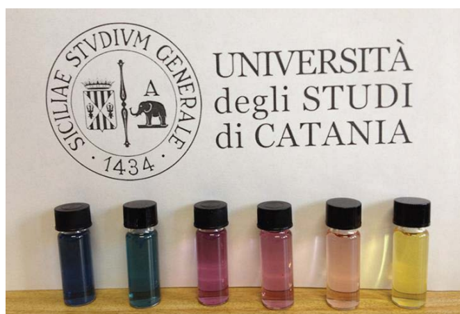
Figure 7: Various silver nanoparticles at different plasmon resonance
