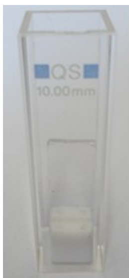
Figure 2.2.6. Set-up for UV-Vis measurements of the quartz substrate bearing a porphyrin monolayer.
