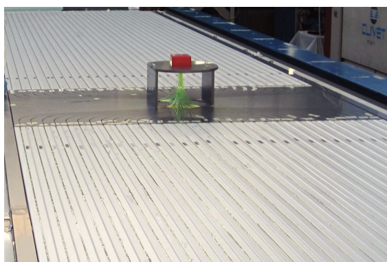
Figure 4.2: The fiber router and the optical connector. The protective dome has been removed.
