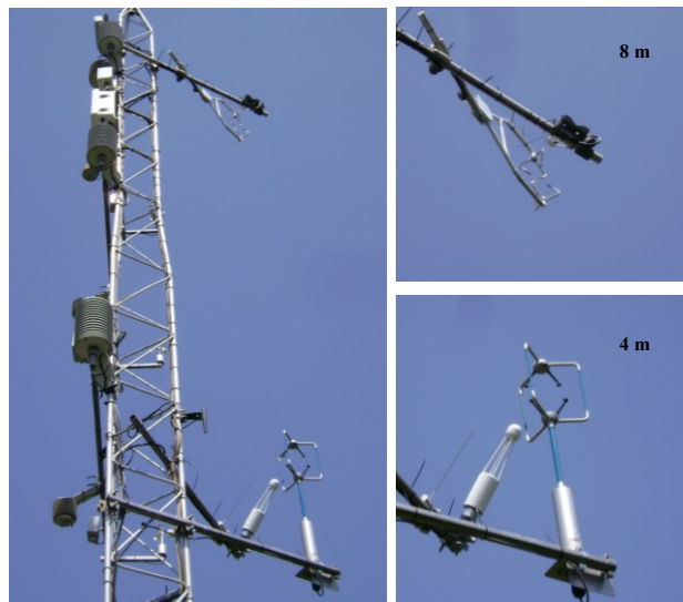
Fig. 6.6. The two levels for SR and EC measurements.
