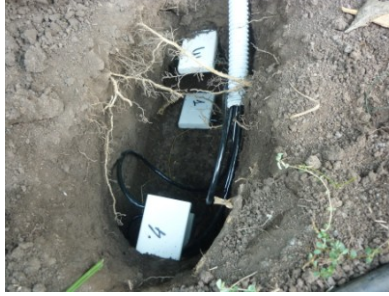
Fig. 6.8. TDR probes into the soil.
