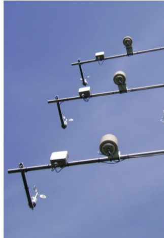
Fig. 6.7. Temperature, humidity and wind profile.
