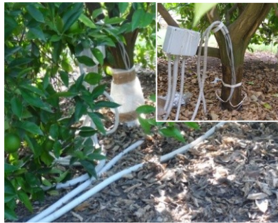
Fig. 6.9. HPV probes installed for Sap Flow measurements.
