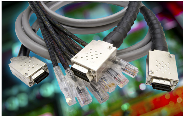
Figure 4.21 - MRJ21 cables 15 m long (on the left). National Instrument cables SHC68-68-RDIO (on the right).
