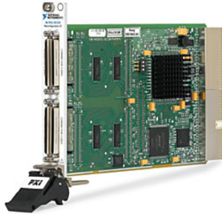
Figure 4.19 - National Instrument PXI- 7813R with 160 digital I/O.
