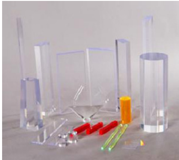
Figure 1.6 - Plastic scintillators of different shapes, colours and sizes.
