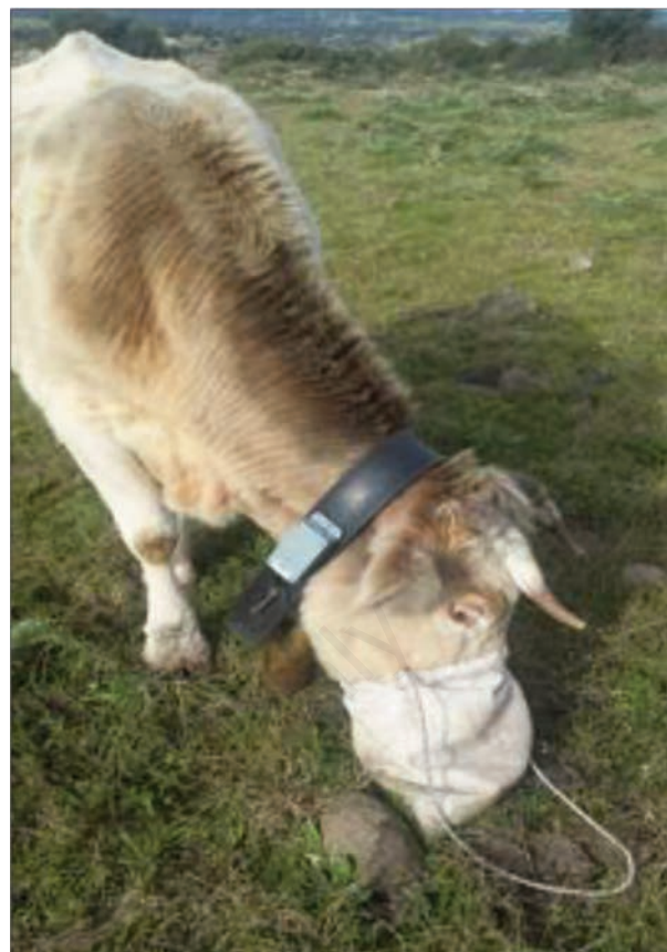
Figure 3. Low power-global positioning system device attached to the cow's collar.
