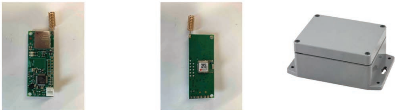
Figure 6. Low-power global positioning system device and the IP case.
