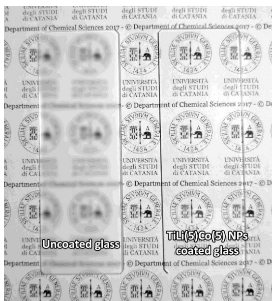
Fig. 69: Comparison of antifogging properties between uncoated (left) and TiLi(5)Co(5) NPs coated glass slide in steamed environment
