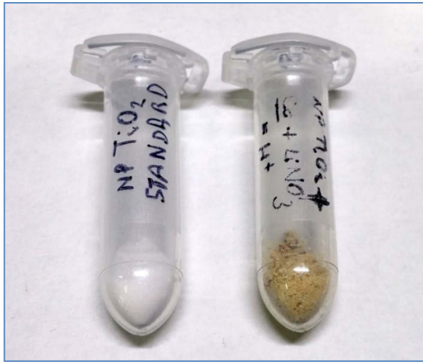
Fig. 21: Samples of nanoparticles of ND- \text{TiO}_2 (left) and \text{TiLi}(5)\text{Co}(5) (right).
