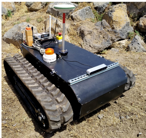
Figure 4.17 The U-Go robot adapted for teleoperation missions
