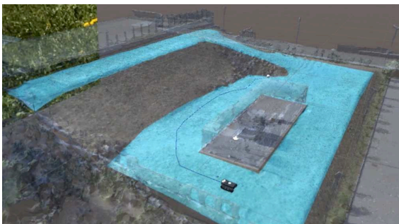
Figure 4.12 The traversable area represented as a cyan layer overlaid onto the environment model reconstruction
