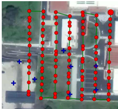
Figure 3.1 Example of back-and-forth motion for aerial imagery acquisition (pictures position represented as red circles)
