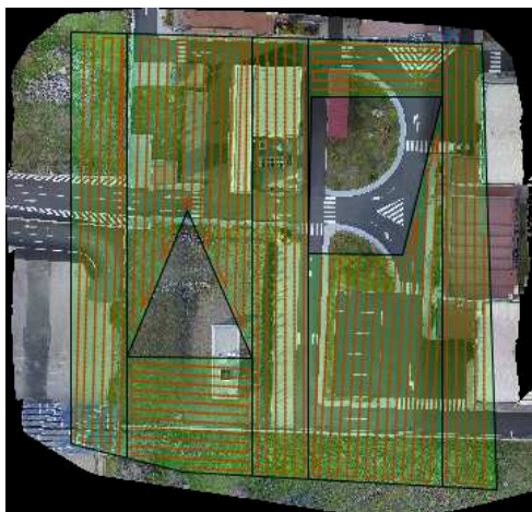
Figure 5.5 Example of environment decomposition with optimal coverage trajectories
