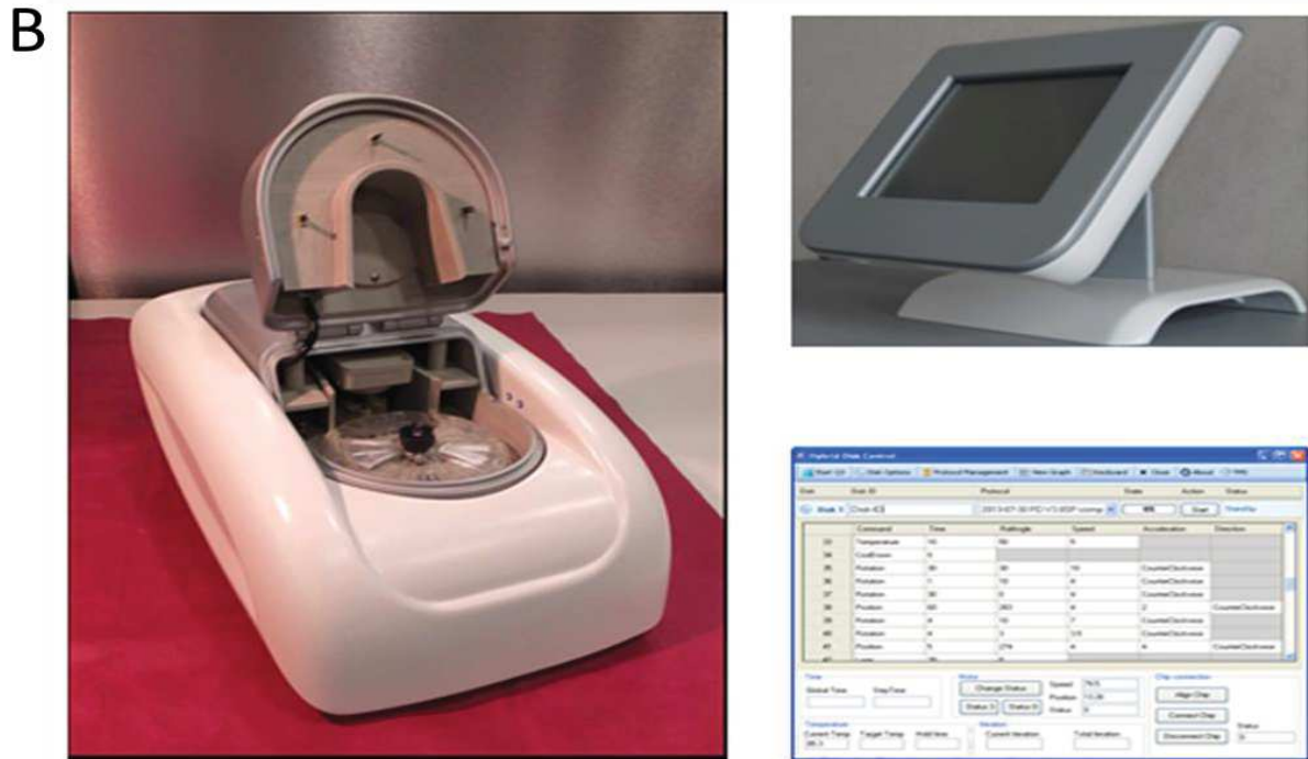
Fig.4. DNA-disk platform (A) Hybrid disk: sample prep + polycarbonate disk + Real Time PCR chip (yellow ring). (1) Sample loading chamber; (2) lysis chamber; (3) washing chamber I; (4) washing chamber II; (5) DNA elution and collection chamber; (B) P1B player and software.
