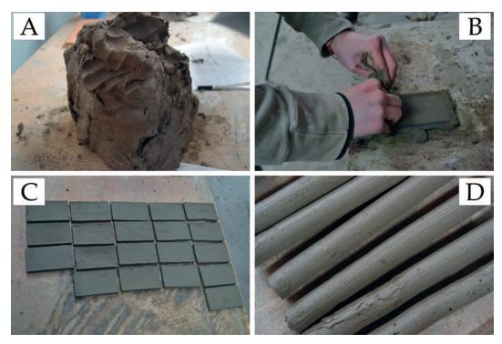
Figure 2. Manufacture of ceramic test-pieces: (A) example of experimental paste at the "green state"; (B) manufacturing experimental briquettes by means of customized wooden-framed mould; (C) ceramic briquettes during the air dry phase; (D) ceramic cylinders during the air dry phase.
