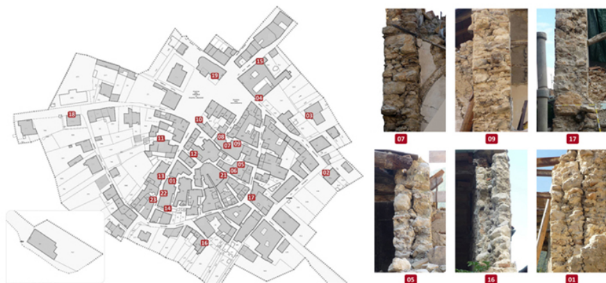
Figure 7 – Villa Sant'Angelo, masonry works analysis
