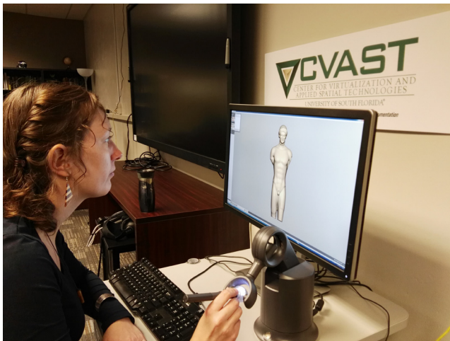
Fig. 26 Touch interaction with the digital model of the statue through haptic technology.
