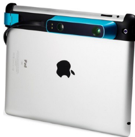
Fig. 8 Structure sensor clipped onto an iPad.
