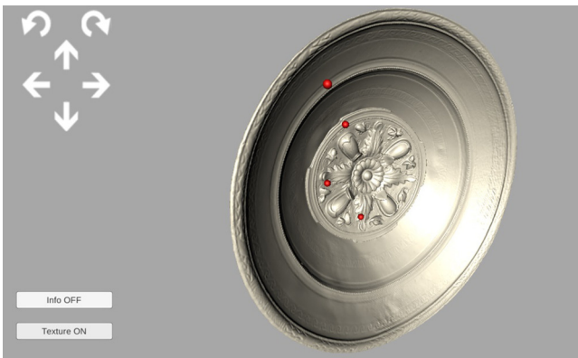
Fig. 23 Shaded version of a 3-D model in Unity platform. Red spheres are used as markers.
