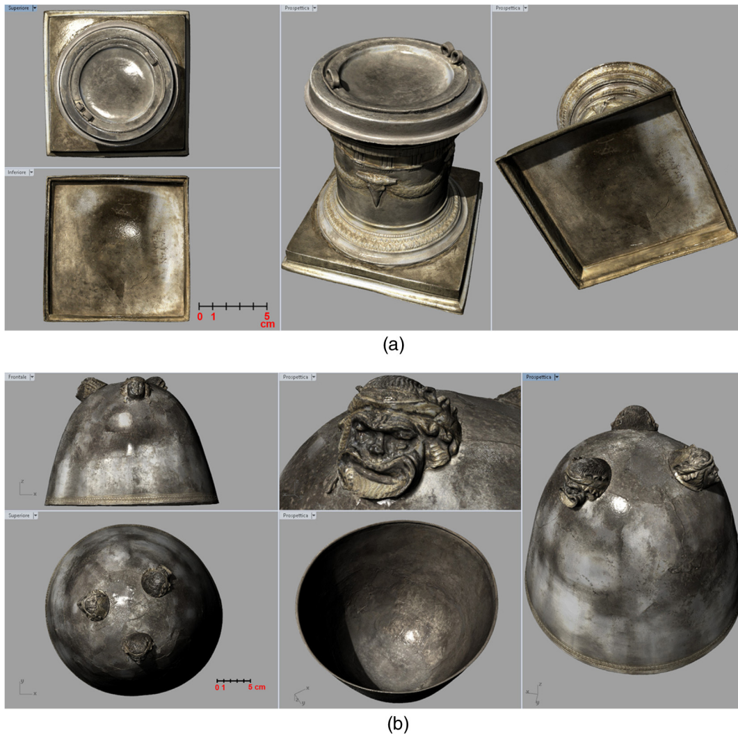
Fig. 10 Orthogonal and perspective projections: (a) the arula and (b) one of the kyathos.
