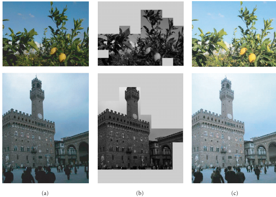
FIGURE 10: Experimental results by postprocessing: (a) original color input image, (b) contrast and focus visually significant blocks detected, and (c) exposure-corrected image obtained from RGB image.
