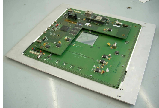
Figure 2: photograph of the tracker module. The L-shaped digital board sits on top of the front end board. The silicon sensor is placed on a squared hole in the center of the latter.
