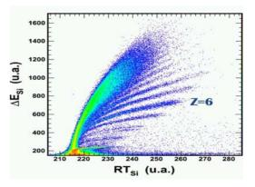
Fig. 2.  $\Delta E$  - Rise Time plot for <sup>78</sup>Kr+<sup>40</sup>Ca , at  $\theta = 34^{\circ}$ .
