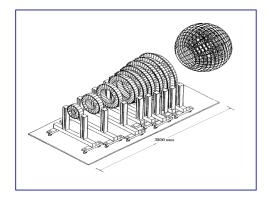
Fig. 1. Sketch of the CHIMERA detector
