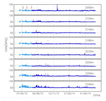
Fig. 12 Baseline rate measured for the whole operation period of the tower at different depths. All selected PMTs are down-looking. *Light blue dots* correspond to the commissioning period of the detector. The *arrows* indicate the dates when PMT high voltage adjustments were performed
