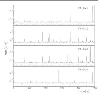
**Fig. 16** Singles rate as measured in the monitoring channel of the four OMs of the 1st floor as a function of time for a 1000 s time slot measured on July 11 2013, corresponding to a period of relatively high-level bioluminescence activity (same as the one shown in Fig. 11a)
