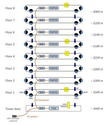
**Fig. 6** Schematics of the NEMO Phase-2 tower, including the backbone cabling (*orange*), the Floor Module Protective Oceanic Device (FMPOD) and the electro-optical breakouts (BoB). Connection to the Junction Box is provided through a ROV-mateable hybrid connector, installed in the tower base. The position of the environmental probes are also indicated as well as those of the hydrophones (H0 and H1) (see text for details). Nominal depths of each floor are given on the *right*
