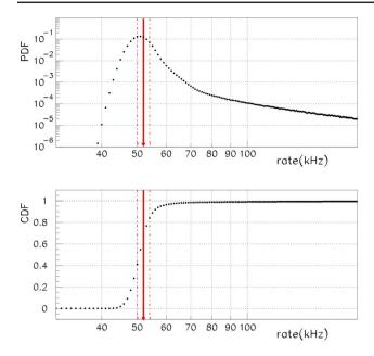
**Fig. 15** Probability Density Function (PDF) and Cumulative Density Function (CDF) of singles rate (*black dots*) for the whole set of data taken from July 2013 to August 2014 of one PMT. The *solid red line* indicates the result of the GEANT4 simulation described in the text. *Dashed red lines* give the error in this simulation
