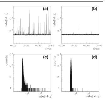
Fig. 11 Singles rate as measured in the monitoring channel as a function of time for 1 h time slots measured on July 11 2013 (*panel a*) and on September 11 2013 (*panel b*). *Panels c*, *d* show the corresponding histograms of the monitored rate values
