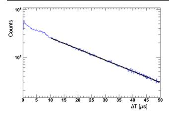
Fig. 10 Time difference between two consecutive hits. The exponential fit above  $\Delta t = 10 \,\mu s$  (*black line*) gives a characteristic time  $\tau = 1.8 \times 10^{-5}$  s. The bump at  $\Delta t \approx 7 \,\mu s$  is due to the presence of PMT afterpulses. For  $\Delta t < 1 \,\mu s$  the effect of electronics deadtime is present
