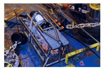
Fig. 3 An image of Cable Termination Frame on the ship deck prior to its deployment
