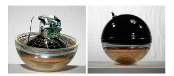
**Fig. 7** *Left* One hemisphere of the optical module glass vessel containing the photomultiplier and the front-end module board. *Right* An optical module fully integrated with the electro-optical feedthrough and the pressure-meter
