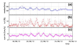
**Fig. 17** a Baseline rates over a 15 min period; b burst fraction (b.f.), defined as the fraction of time in the 15 min window with rate exceeding 100 kHz; c modulus of the water current velocity measured with the DCS
