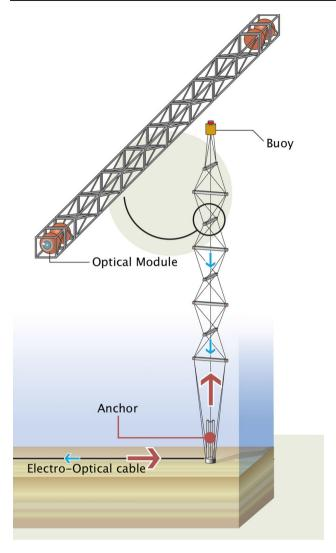
Fig. 4 Sketch of the NEMO Phase-2 tower. The structure is formed by a sequence of eight floors, each one supporting four optical modules. The structure is anchored at the seabed and kept taut by a buoy located at the *top*. *Vertical* distances are not to scale
