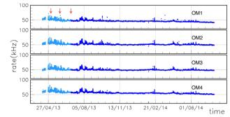
Fig. 13 Baseline rate measured for the whole operation period of the tower for the four OMs of the 1st floor of the tower. The OM numbering follows the scheme illustrated in Fig. 6 with OM 1 and 4 that are horizontally looking and OM 2 and 3 downward looking. *Light blue dots* correspond to the commissioning period of the detector. The *arrows* indicate the dates when PMT high voltage adjustments were performed
