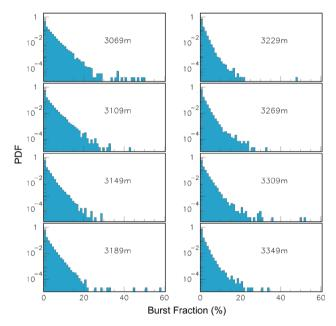
**Fig. 14** Probability Density Function (PDF) of observing a given burst fraction, defined as having a rate exceeding 100 kHz in a 10 ms time window, in eight down-looking OMs placed at different depths
