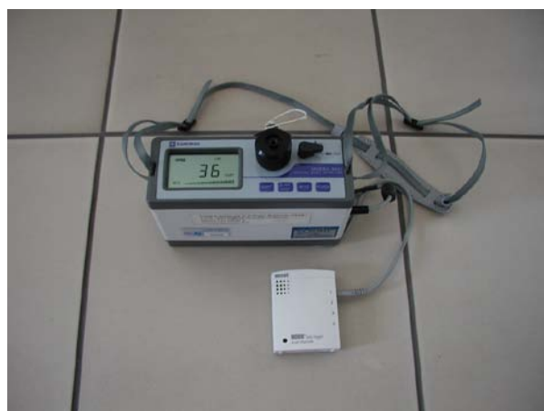
Figure 2. Dust monitor and data logger unit.
