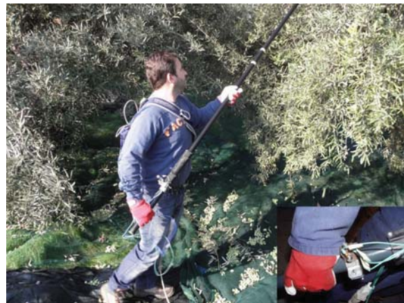
Figure 2. Positioning of the accelerometers on the bar.
