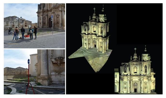
Fig.8: St. Antonio Church, Ferla: laser scanner surveying and digital data post processing.
