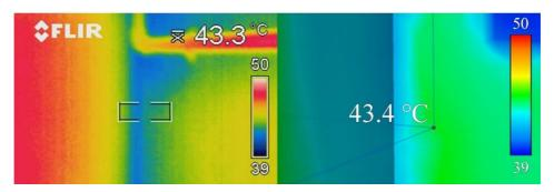
**Figure 10.** Comparison between data obtained by using the thermal camera and data simulated by CFD analysis at the north wall.
