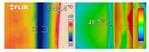
**Figure 12.** Comparison between data obtained using the thermal camera and data simulated by CFD analysis at a pillar of the south wall.
