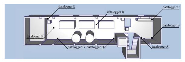
Figure 3. Positions of data-loggers used for the monitoring of indoor air temperature.
