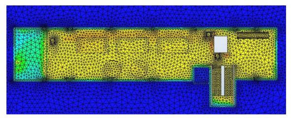
Figure 4. Automatic mesh sizing.
