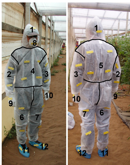
Figure 3. Coverall elements to measure the dermal operator exposure. (1) hood, (2) right arm, (3) left arm, (4) chest, (5) back, (6) right leg, (7) left leg, (8) dust mask, (9) right hand, (10) left hand, (11) right foot, (12) left foot.
