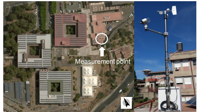
Figure 1. a) View of the investigated area; b) LSI Lastem weather station
