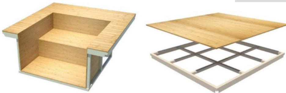
Figure 7. Panel-staircase and axonometric exploded view of the floor panel.
