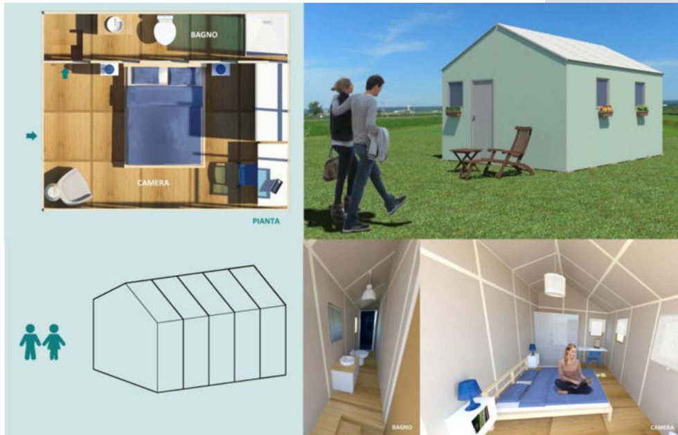
Figure 8. Six-section combination for two people with bathroom.
