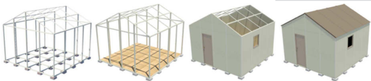
Figure 4. Assembly phases of construction elements.
