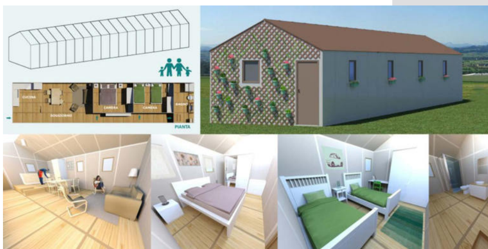
Figure 10. Eighteen section combination addressed to family, with bathroom and living room.
