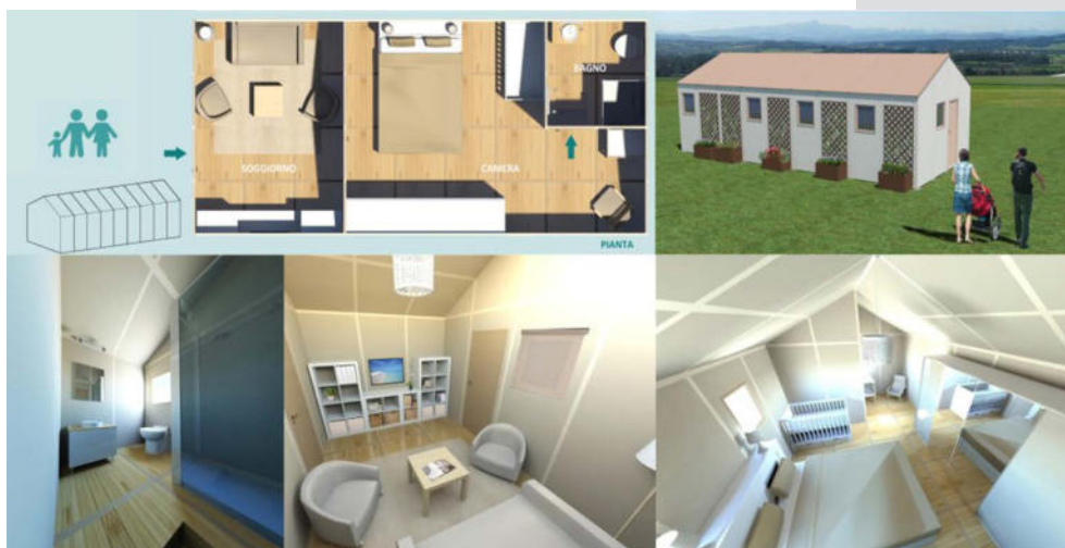
Figure 9. Nine-section combination addressed to family, with bathroom and living room.
