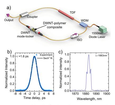
Figure 9. (a) Laser setup at  $\sim$ 2  $\mu$ m. TDF, thulium-doped fiber. (b) Second harmonic generation autocorrelation trace of mode-locked pulses at  $\sim$ 2  $\mu$ m. (c) Output spectrum.
