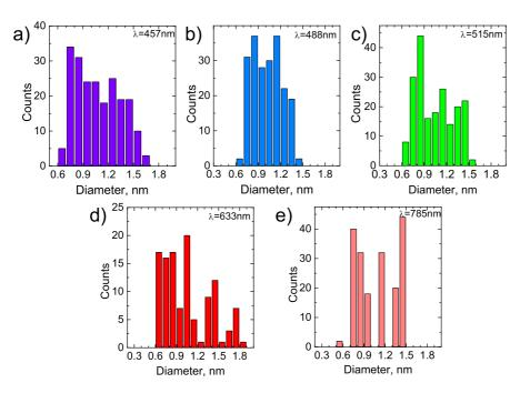
Figure 5. Diameter analysis from the RBMs of the nanotubes excited by (a) 457, (b) 488, (c) 515, (d) 633, and (e) 785 nm wavelengths, indicating  $d_t \sim 0.6-1.8$  nm.
