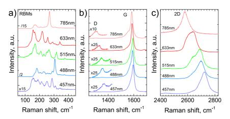
Figure 4. Raman spectra of DWNTs at different excitation wavelengths: (a) RBM region, (b) G region, and (c) 2D region.
