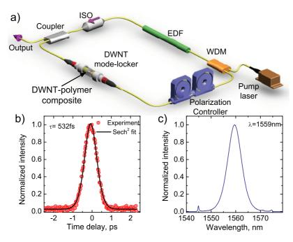
Figure 8. (a) Laser setup at 1.5  $\mu$ m. EDF, erbium-doped fiber; WDM, wavelength division multiplexer. (b) Second harmonic generation autocorrelation trace of mode-locked pulses at 1.5  $\mu$ m. (c) Output spectrum.
