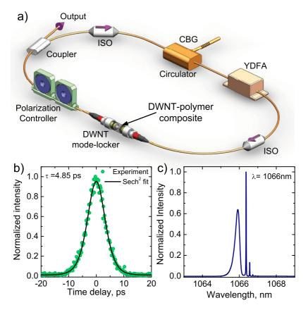
Figure 7. (a) Laser setup at 1  $\mu$ m. ISO, isolator; CBG, chirped Bragg grating; YDFA, Yb-doped fiber amplifier; PC, polarization controller. The DWNT polymer composite is sandwiched between the fiber connectors. (b) Second harmonic generation autocorrelation trace of the output pulses at 1  $\mu$ m. (c) Output spectrum.
