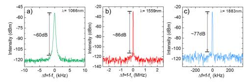
Figure 10. RF spectrum measured around the fundamental repetition rate: (a)  $f_1 = 16.37$  MHz, (b)  $f_1 = 27.4$  MHz, (c)  $f_1 = 17.82$  MHz showing peak to pedestal extinction ratios >60 dB in all three wavelengths.
