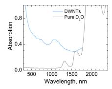
Figure 2. Absorption spectrum of DWNTs dispersed in  $D_2O$  in the 300–1800 nm range. The contribution from  $D_2O$  is subtracted. Spectrum of  $D_2O$  is also presented.
