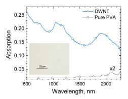
Figure 6. Absorption spectrum of DWNTs embedded in  $\sim$ 50  $\mu$ m PVA polymer composite. The contribution from PVA is subtracted. Absorption spectrum of a pure PVA polymer of the same thickness is also presented. Inset: Optical microscopy of the DWNT-polymer composite reveals no large nanotube aggregation.
