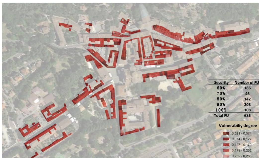
Figure 2. Map of the vulnerability of the Façade Units of the old town of Brisighella. The table classifies the Façade Units by vulnerability degree.
