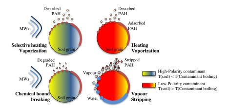
Figure 2: Schematic of PAH removal mechanisms from soil.
