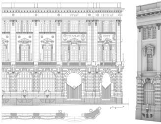
Fig. 5 - Palazzo delle Poste: project drawing of the corner detail (on the left), main facade elevation and 3D model of a facade span (on the right) (2D restitution and 3D model by Biondi R., Cucuzza D., Cutrufo R., Lauria L., Musumarra S., Quaceci N., Ruggieri F., Saitta C., Zammataro C.)
