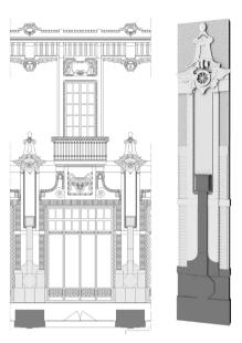
Fig. 8 - Garage Musmeci: project drawing of the plan (on the top), detail of the façade (on the left) 3D model of the parasta (on the right). (2D restitution and 3D model by Ferrara E., Fichera A., Paladina G., Perrone V.)
