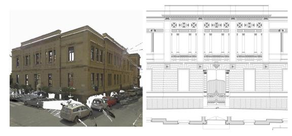
Fig. 3 - Palazzina Enel: view of the point cloud (on the left), main façade elevation (on the right) (2D restitution by Ardito G., Avanzato S., Balba A., Buscemi G., Cosentino S., Frazzetto L., Paganello F., Puccia D., Rapisarda D.)
