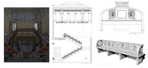
Fig. 4 - Palazzina Enel: view of the monumental staircase point cloud (on the left), cross section of the monumental staircase (center), detail of the bench (on the right) (2D restitution and 3D model by Ardito G., Avanzato S., Balba A., Buscemi G., Cosentino S., Frazzetto L., Paganello F., Puccia D., Rapisarda D.)
