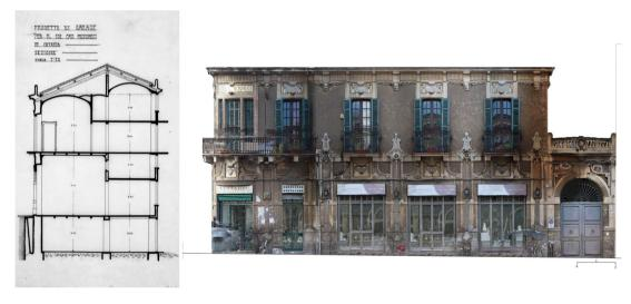
Fig. 7 - Garage Musmeci: project drawing of the cross section (on the left), orthophoto of main façade by poligonal model (on the right) (poligonal model by Ferrara E., Fichera A., Paladina G., Perrone V.)
