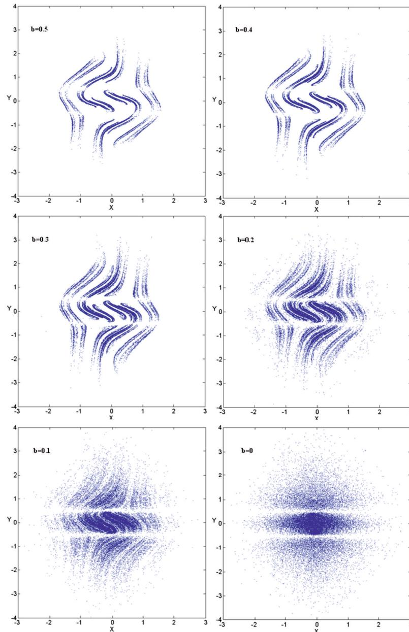
Fig. 12. Experimental cross sections of the trajectories in the  $Z = 0$  plane with  $a = 5$  ( $R_8 = 200k\Omega$ ).
