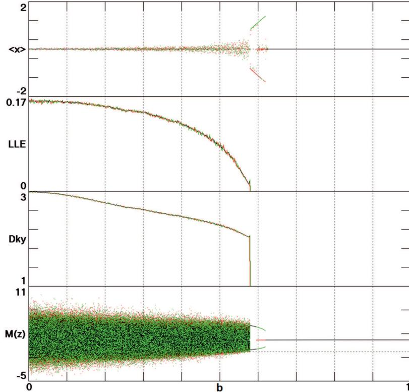
Fig. 6. (From top to bottom) Regions of coexisting attractors ( $\langle x \rangle$ ), the largest Lyapunov exponent (LLE), Kaplan-Yorke dimension ( $D_{KY}$ ), and local maxima of  $z$  ( $M(z)$ ) as a function of  $b$  with  $a = 5$  for Eq. (5).
