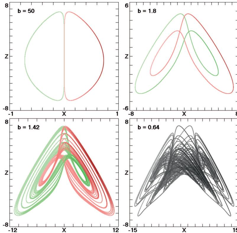
Fig. 4. (a) Trajectories projected onto the  $x$ - $z$  plane of limit cycles for  $b = 50$ , (b) and for  $b = 1.8$ , (c) two coexisting strange attractors for  $b = 1.42$ , and (d) a single strange attractor where the maximum chaos occurs at  $b = 0.64$  for  $a = 5$ .
