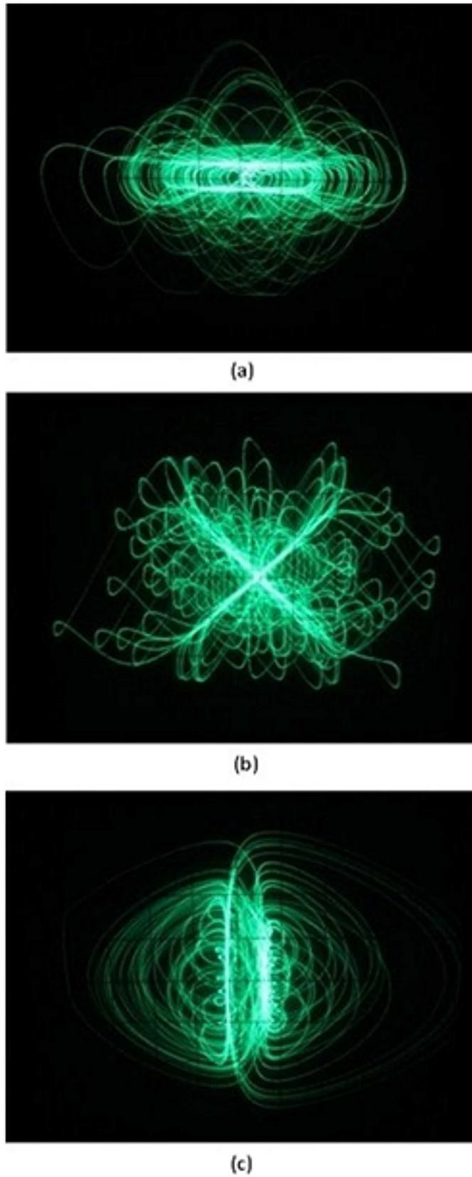
Fig. 11. Oscilloscope traces from the circuit (a)  $X$ - $Y$  plane (b)  $X$ - $Z$  plane (c)  $Y$ - $Z$  plane.
