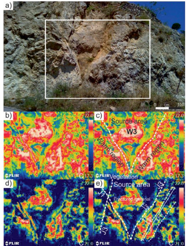
Fig. 5 - WS2 rock mass a) photo taken in daylight, rectangle encloses the area of thermograms; b) thermogram 17.3-22°C, c) thermogram 17.3-22°C with particular elements highlighted; d) thermogram 21-22°C; e) thermogram 21-22°C with particular elements highlighted
