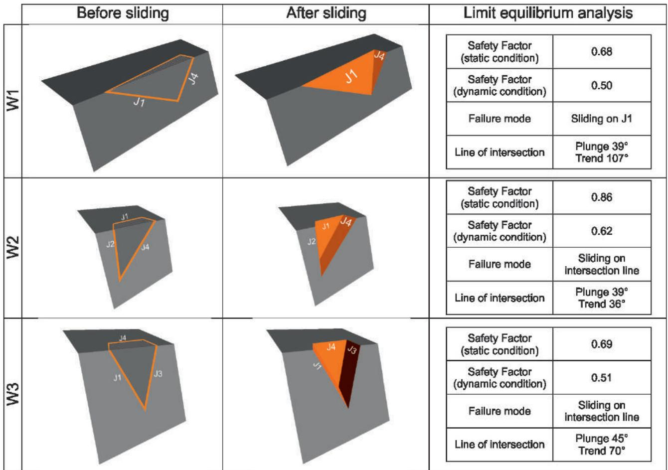
Fig. 3 - 3D models of the main wedges
