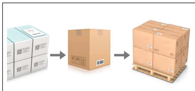
Fig. 2. Serialization and packaging hierarchy (unit box, case box and pallet).
