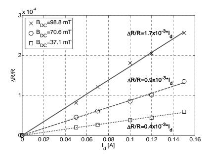
Figure 7. The relative resistance change of the IJP strain gauge as function of the driving current.
