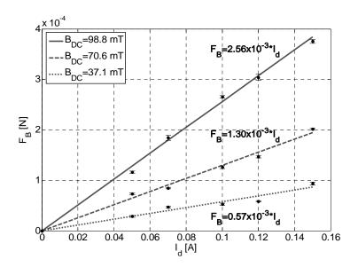
**Figure 5.** The measured force  $F_B$  as a function of  $I_d$  for different values of  $B_{DC}$ .
