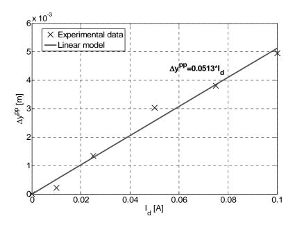
**Figure 9.** The device response in case of sinusoidal driving current @4.1 Hz and  $B_{DC}$  = 37.1 mT.
