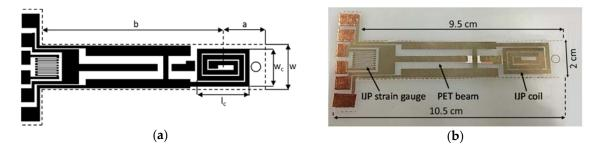
**Figure 2.** The IJP actuator. (a) Layout of the inkjet printed coil and strain gauge; (b) real view of the device.
