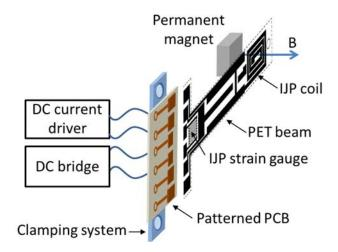
Figure 1. Schematization of the Inkjet Printing (IJP) actuator.
