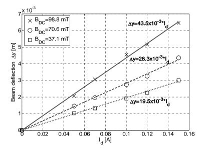
Figure 6. The beam deflection as function of the driving current.
