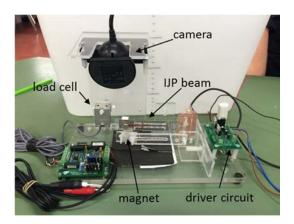
Figure 4. The experimental setup.
