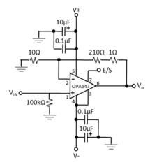
Figure 3. The electronics for the electromagnetic driving mechanism.
