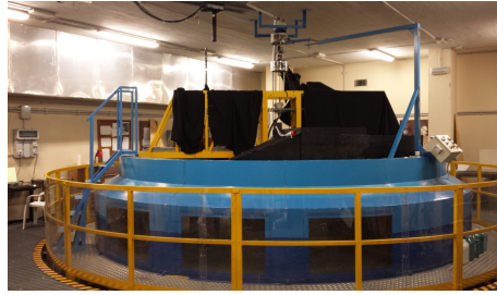
Figure 1: The TurLab rotating tank. The black tube on the ceiling is the collimator of the experimental set-up used to mimic the JEM-EUSO telescope.
