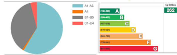
Fig.8. Embodied carbon by life-cycle stage and Embodied carbon benchmark
