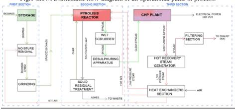
Fig.1 shows a schematic flow-diagram of all operational paths of process.
