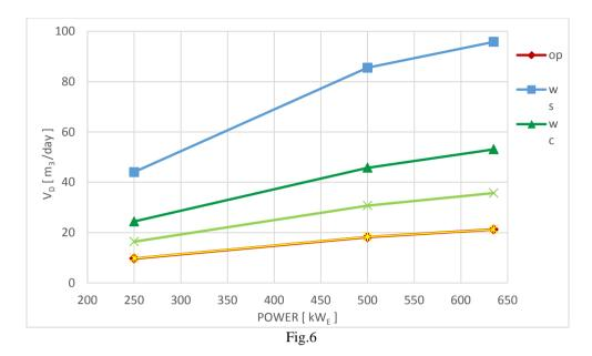
The pattern of Fig.6 allows a rough valuation of  $v_d$  also for powers not strictly corresponding to that ones investigated.
