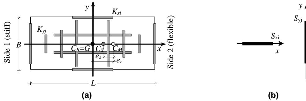
**Fig. 3 – Analysed single-storey systems: (a) Plan layout of the systems; (b) uni-directional resistance of the resisting elements**
