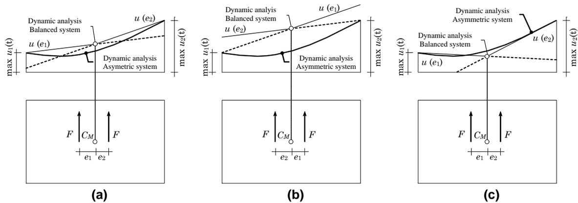
**Fig. 1 – Envelope of dynamic displacements vs. displacements determined by the nonlinear static method and corrective eccentricities: (a)  $U_{CM,b} > U_{CM,a}$ ,  $e_1 < e_2$ , (b)  $U_{CM,b} > U_{CM,a}$ ,  $e_1 > e_2$ , (c)  $U_{CM,b} < U_{CM,a}$**
