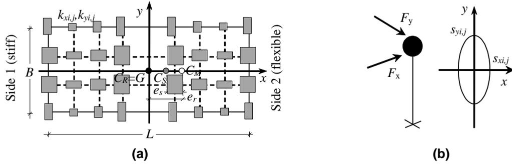
**Fig. 2 – Analysed single-storey systems: (a) Plan layout of the systems; (b) bi-axial yield domain of the resisting elements**
