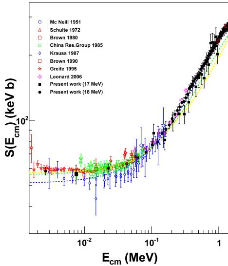
**Figure 1.** S(E) factor for the  ${}^2\text{H}(\text{d},\text{p}){}^3\text{H}$  reaction: black solid squares and circles are THM data (17 and 18 MeV respectively); colored symbols represent direct data as described in the legend.
