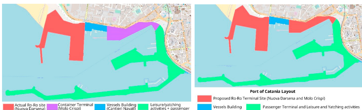
Fig 6. Port of Catania Layout: (a) actual configuration and (b) proposal
